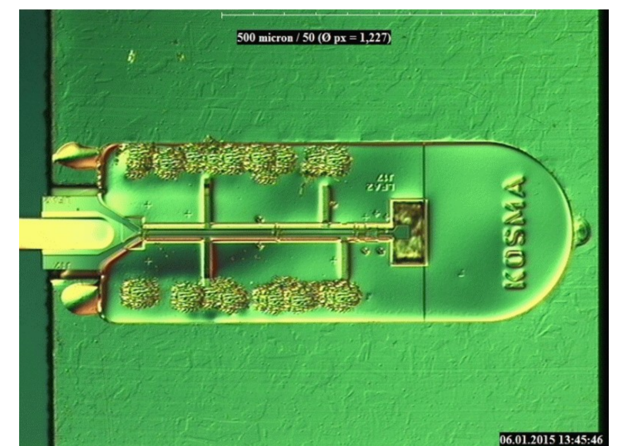
FIGURE 5: Two-Microscope photograph of a 2.0THz HEB device mounted on its waveguide block developed for upGREAT. The actual device is seen right of the center of the image. The conical shaped waveguide probe antenna can be recognized by eye. The HEB microbridge left of it is not visible at this resolution (from Pütz et al. 2015).
